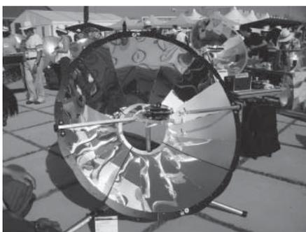
Figure 5 The Japanese take on the SK. Note the high quality finishes, legs and pot holder (photo: Marlett Balmer)
