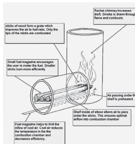
Figure 3 Diagrams showing the principles behind the fuel efficiency in rocket stoves (diagram: Peter Scott)
