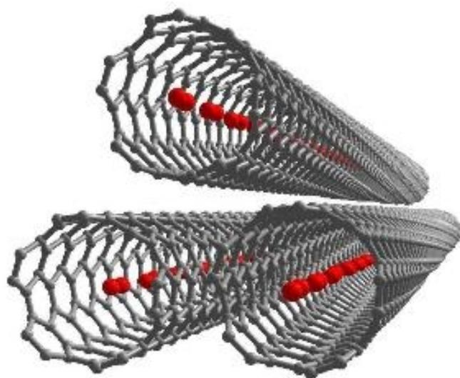
**Figure 3.** Schematic of  $C_{60}$  and  $C_{70}$ -encapsulating carbon nanotubes incorporation into the Nano Polymeric Matrix (NPM) by immersion of the Nano Polymeric Modified Electrode (NPME)
