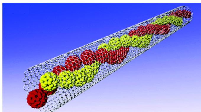
**Figure 1.** Simulation of C<sub>60</sub> and C<sub>70</sub>-encapsulating carbon nanotubes incorporation into the Nano Polymeric Matrix (NPM) by immersion of the Nano Polymeric Modified Electrode (NPME)
