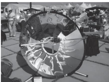
Figure 5 The Japanese take on the SK. Note the high quality finishes, legs and pot holder (photo: Marlett Balmer)
