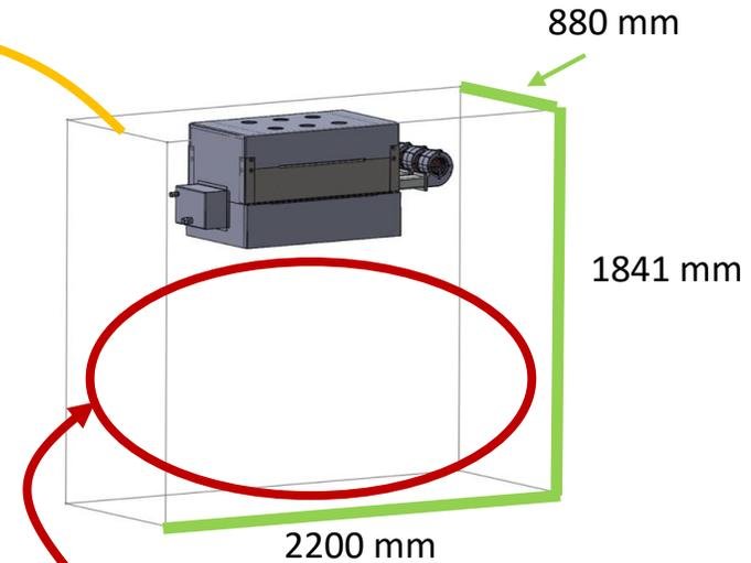
Space for 2,200 L methanol/water tank (equiv. to 190 kg H<sub>2</sub>)
