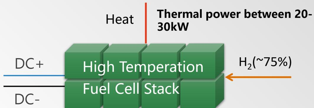
We use “high-temperature fuel cell stack” , the temperature of the heat exchanger is about 140 degrees, the heat energy can be fully utilized to heat the lithium cell and the car.
