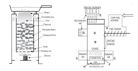
Figure 1 Diagrams of a forced-air TLUD, left, and an AVUD micro-gasifier, right. (*diagram: Tom Reed, left, and Chip Energy, right.*)
