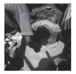
Figure 8 Final touches are given, the inside of the stove is smoothened and cleaned. (*photo: Peeyush Sekhsaria*)
