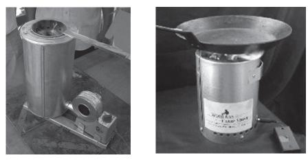
Figure 2 Reed's Woodgas Campstove (left) for sale on the Internet (US\$55) and Anderson's Juntos B+ TLUD gasifier (with removable fuel canister) hand-made in Cambodia with GERES (estimated cost under US\$20). For cooking, the pot can be placed on top of the unit or (better) be positioned on a simple pot support structure of any size so that the gasifier can be moved for refilling without disturbing the pot. (*photos: Tom Reed, left, Paul Anderson, right*)
