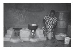
Figure 5 Two maendeleo liner installed (*photo: Anna Ingwe*)
