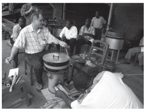
Figure 1 Testing of a commercially manufactured Rocket Stove from Uganda, at GTZ Technical Workshop in Mulanje, Malawi (*photo: Elmar Dimpl*)
