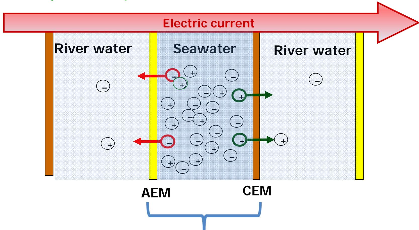
Each pair of seawater + river water cells  $\rightarrow$   **$\sim 0.1 - 0.2$  V**
