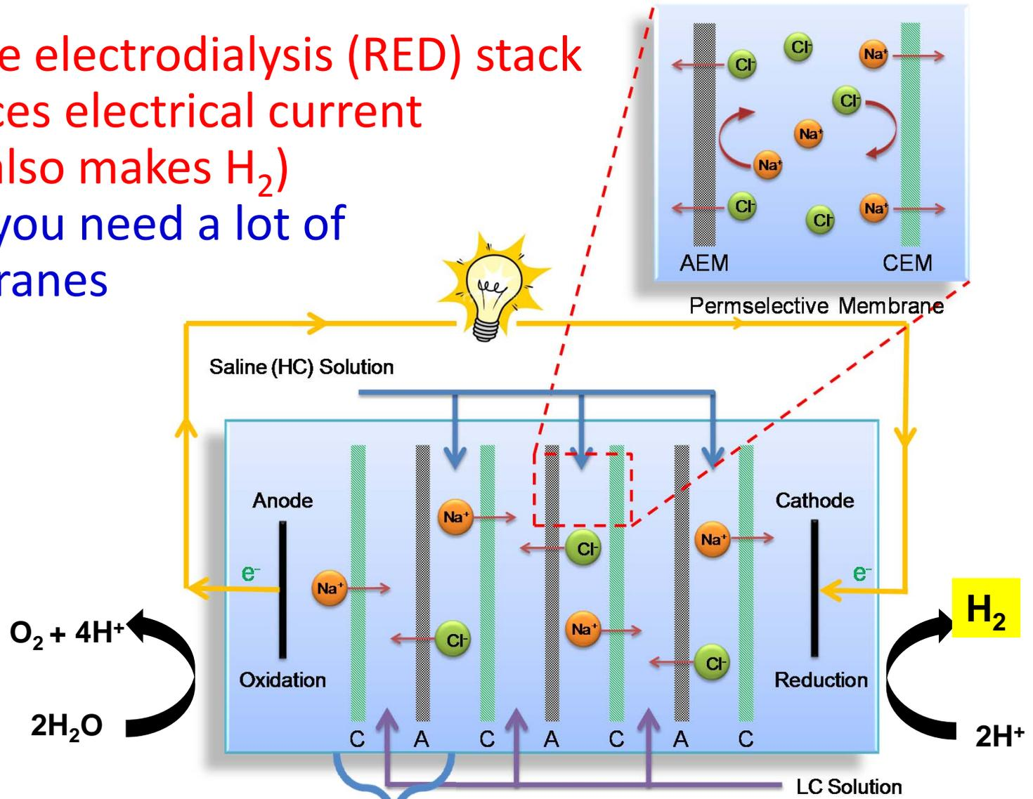
Each pair of high salt (HC) + low salt (LC) cells =  $\sim 0.1 - 0.2 \text{ V}$
