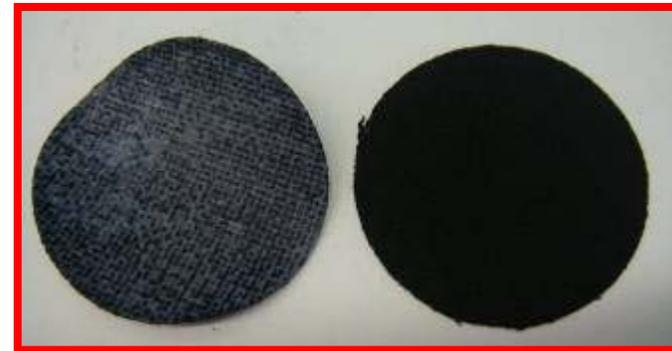
Activated carbon cathode works almost as well as Pt catalyst
