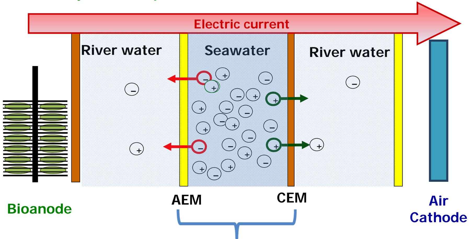
Each pair of seawater + river water cells  $\rightarrow$   $\sim 0.1 - 0.2$  V
