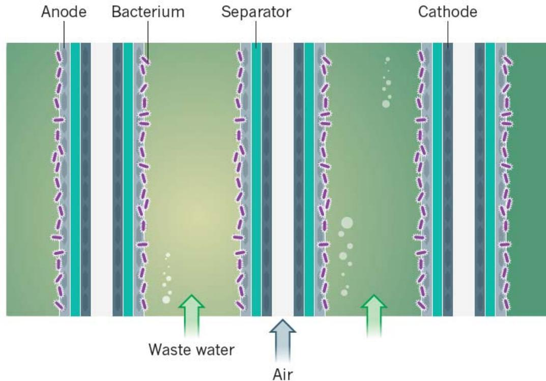
**Figure 3 | An MFC stack.** MFCs are arranged close together to reduce internal resistance and form compact reactors. Within the stack the electrodes consist of repeating units of an anode coated in a mat of bacteria, or biofilm, an insulating separator and a cathode. Waste water flows over the anodes and air over the cathodes. The individual anode and cathode are connected by a wire (not shown).
